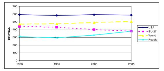
Figure 3. CO2 emissions intensity of electricity and heat output
